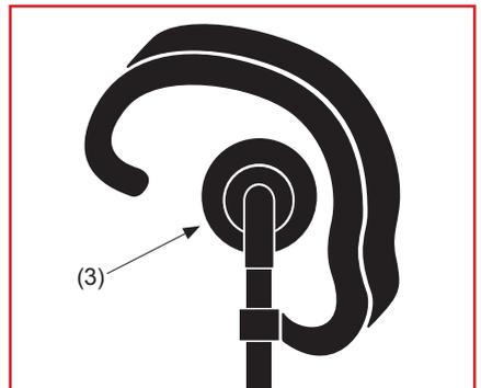
The accessory of the Comfort Ear-Bud with Ear-Hook can be changed easily. Therefore you just need to pull off the black foam cover (3) and exchange it.
