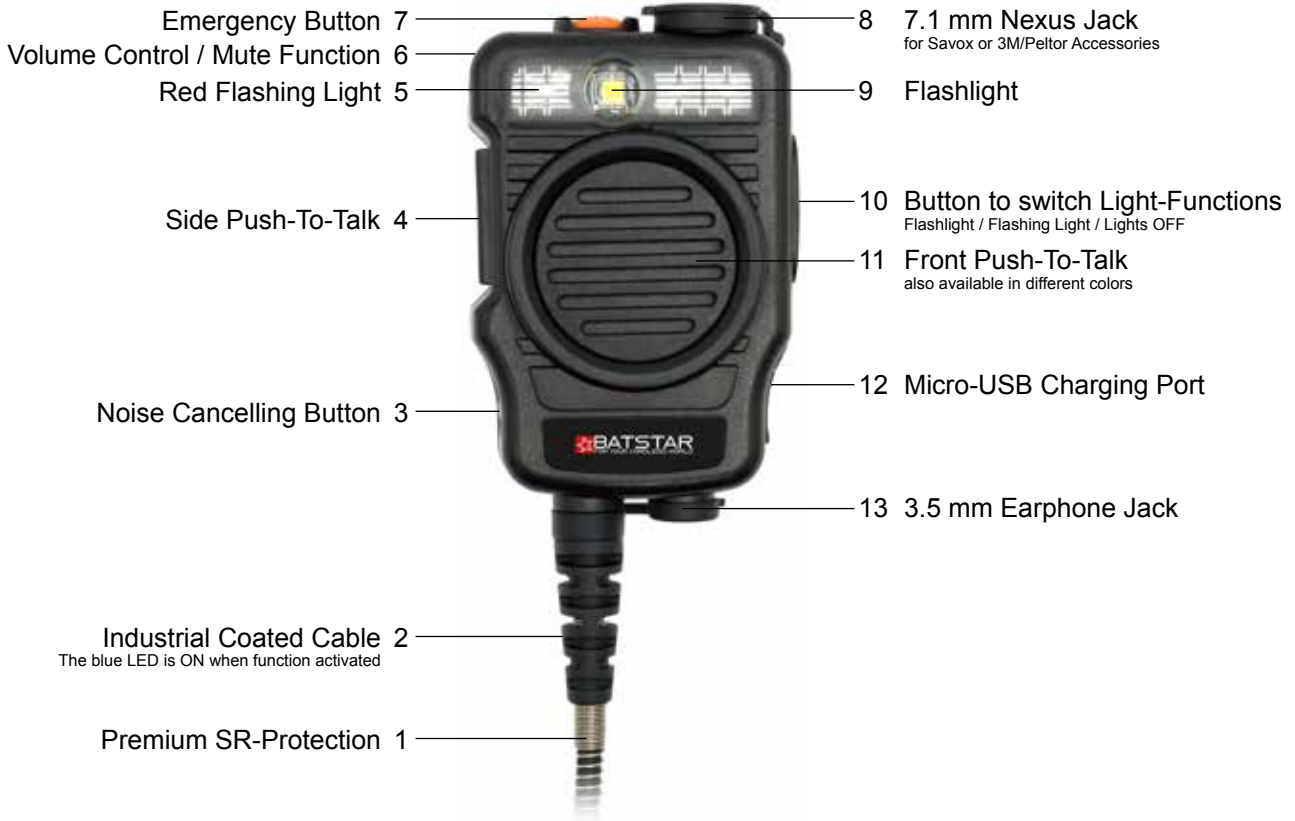
Multi-Function Speaker Microphone (IP67) with 360° Clip, 3.5 mm Audio Jack, 7.1 mm Nexus Jack for Savox, Noise Cancelling Microphone, Emergency Button, Volume Control, Reflective Board & Megaphone Function for Sepura
